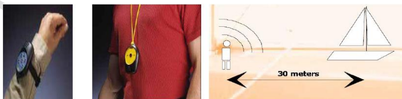
Man Overboard Detection System (NKY, accessed 2016)
